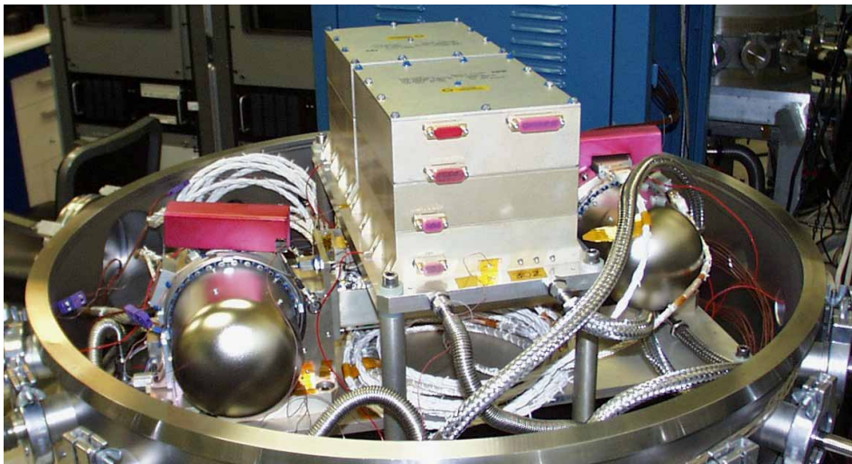
FIGURE 7. TES coolers and electronics during performance characterization testing at JPL.
