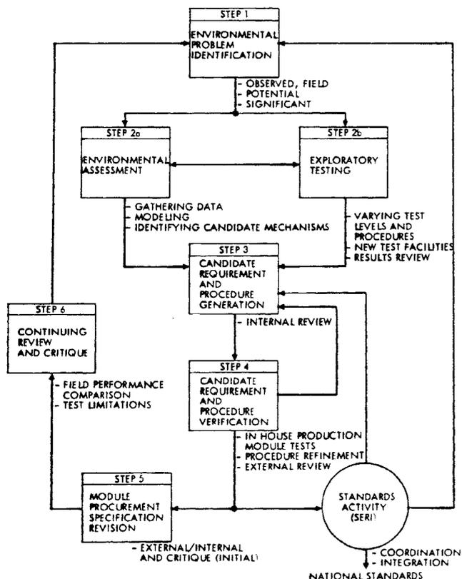
Figure 1. Flow diagram of approach for developing environmental qualification test requirements and procedures for flat plate solar cell modules
