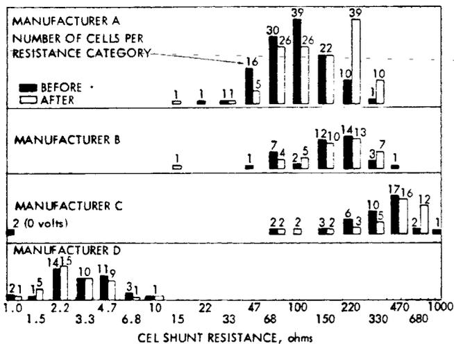
Figure 7. Cell shunt resistance before and after bias humidity testing
