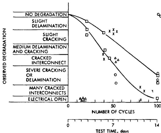
Figure 3. Observed temperature cycling degradation
