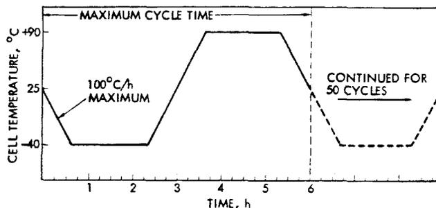
Figure 2. Temperature cycling test profile
