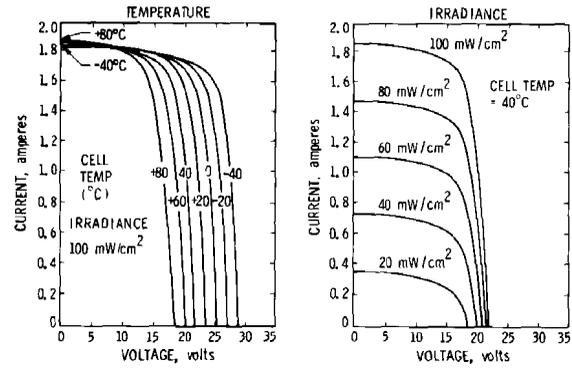
Fig. 2 - Typical silicon photovoltaic module temperature/irradiance-level dependence
