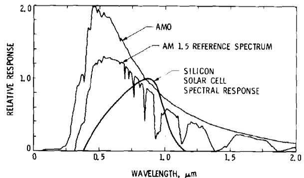
Fig. 1 - Typical solar cell spectral response versus two solar irradiance spectra
