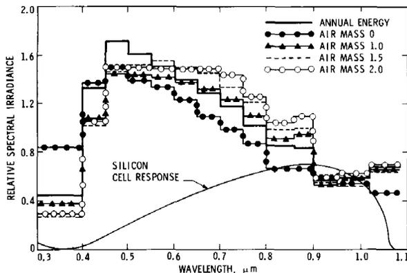
Fig. 5 - Comparison of terrestrial spectra with AM 1.5 reference spectrum normalized for equal total irradiance
