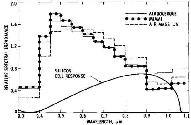
Fig. 4 - Comparison of annual irradiant energy spectral distributions with AM 1.5 reference spectrum normalized for equal total irradiance
