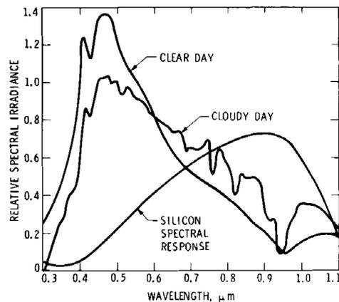
Fig. 3 - Typical diffuse sky spectral distributions normalized for equal total irradiance
