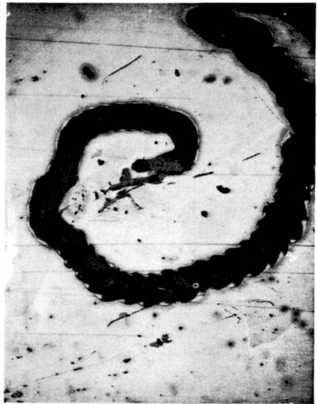
Figure 12. Wormlike Metallization Loss Pattern on Q-Si Module A690E, 40X
