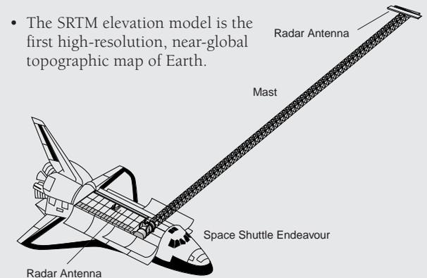
*SRTM simultaneously used antennas in the payload bay and at the end of a mast to record radar signals reflected off Earth's landforms from two differing viewpoints.*
