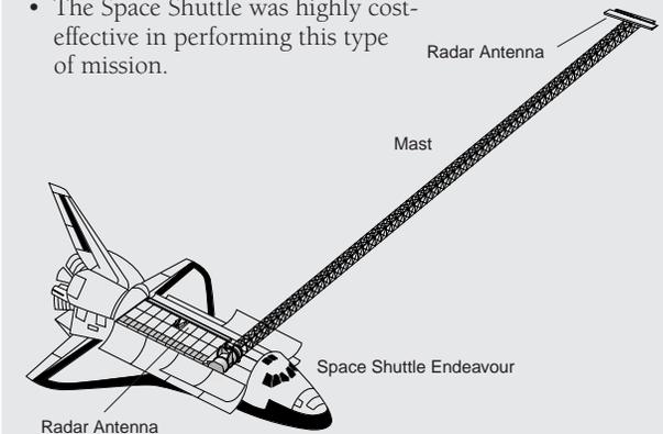
SRTM simultaneously used antennas in the payload bay and at the end of a mast to record radar signals reflected off Earth's landforms from two differing viewpoints.
